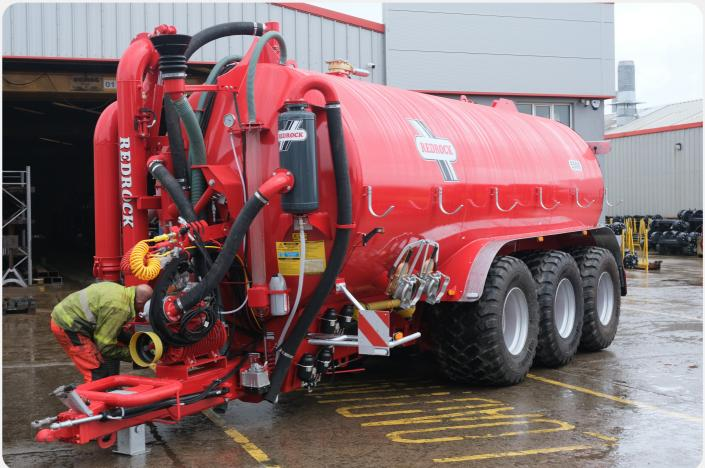
For the toughest jobs, you need the toughest tankers. The Redrock Tri Axle tanker range is designed with strength and longevity in mind, along with optimum performance and maneuverability. With a 1 degree loading angle, efficient emptying of the tank is easily accomplished. Load carrying capacities are available from 5000 UK Gal. (6000 US Gal.) to 8330 UK Gal. (10,000 US Gal.).
