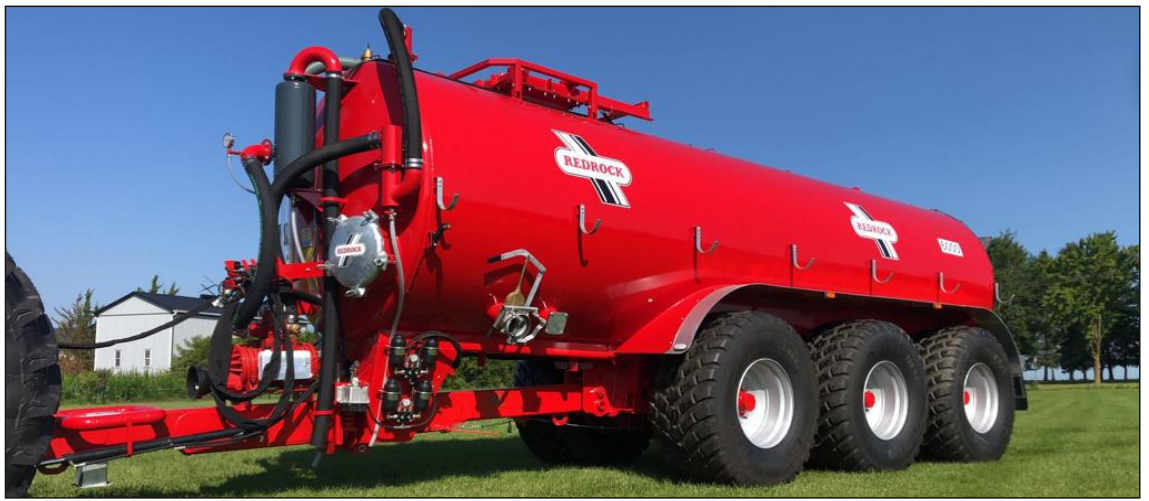
6000 UK Gal (7200 US Gal) Tri Axle Manure Tanker on 750/60 x 30.5 Wheels
