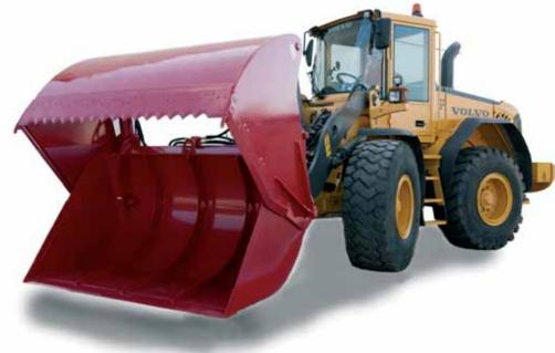
The Redrock 130 Series All Round is suitable for larger industrial wheeled loaders offering unrivalled capacity.
