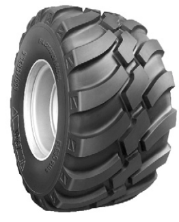
710/50 x 26.5 BKT Radial Width - 710 (28.5") Diameter - 1400 (55")
