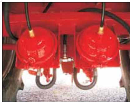
Air/Hydraulic Brake System
